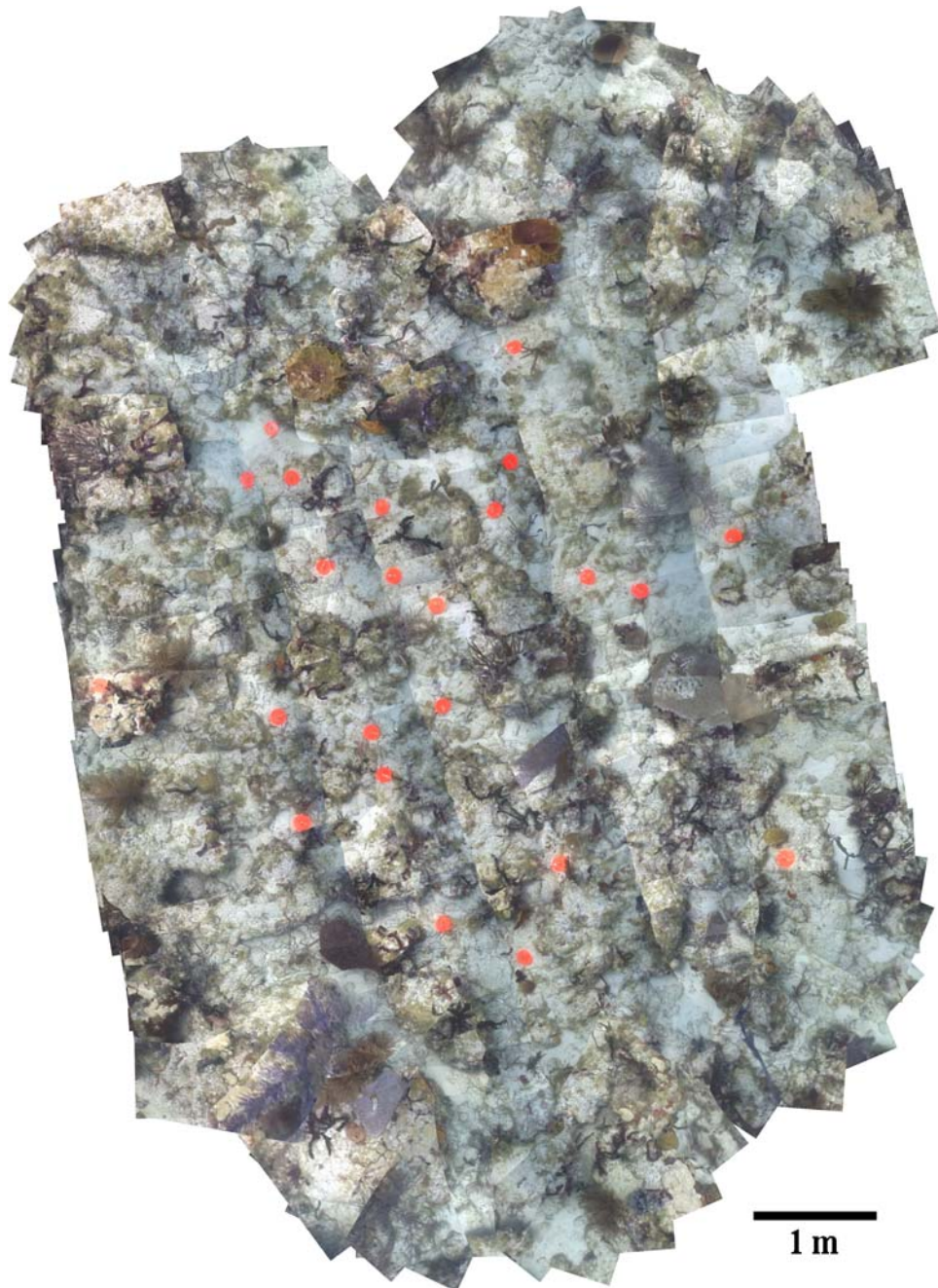
Fig. 3 Video mosaic constructed with video collected from a hand-held digital camcorder in June 2004 at Brooke's Reef in the Florida Reef Tract (depth 7–10 m). The video was collected
